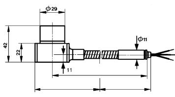
Min. bending radius: 50 mm Clipping points of the cable should be no more than 100 to 200 mm apart
