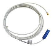
For probe lengths not listed, double the probe's desired physical length in inches and substract from 180 in. for a 15 ft. system or from 240 in. for a 20 ft. system to get the correct extension cable length.
